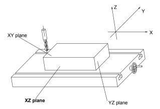
In horizontal plane, the X axis is parallel with the operator; Y axis is perpendicular to X axis. Z-axis is perpendicular to horizontal plane. Positive direction of axis is set as the figure. It also can be changed as customer.
