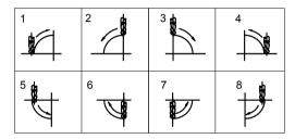
Tool compensation direction (when process XY plane)
