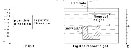
VM600-E provides fireproof function. During EDM, charcoal will be produced on the machined surface. With accumulating charcoal, the electrode will beyond liquid level, which could lead a fire. If fireproof height is set, EDM will stop, the DRO will send an alarm and fire is avoided.
